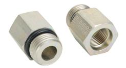
HY-TECH hydraulic fluid adapter, straight, plated steel body, (1) -8 male o-ring boss and (1) -6 female o-ring boss. Package of 2.
