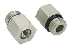
HY-TECH hydraulic fluid adapter, straight, plated steel body, (1) -8 male o-ring boss and (1) -4 female o-ring boss. Package of 2.
