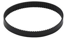
SureMotion timing belt, 0.08in MXL pitch, 1/4in wide, 88 tooth, 7in pitch length (circumference), polyurethane, polyester reinforced. Package of 3.
