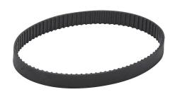
SureMotion timing belt, 0.08in MXL pitch, 1/4in wide, 88 tooth, 7in pitch length (circumference), neoprene, fiberglass reinforced. Package of 3.
