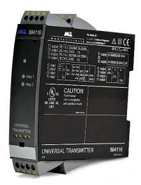
Signal conditioner, isolated, current, voltage, RTD, thermocouple or potentiometer input, deg F or deg C, current, voltage and relay output, 21.6-253 VAC/19.2-300 VDC operating voltage, 35mm DIN rail mount, removable screw terminal plugs.
