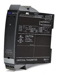
Signal conditioner, isolated, current, voltage, RTD, thermocouple or potentiometer input, deg F or deg C, current or voltage output, 21.6-253 VAC/19.2-300 VDC operating voltage, 35mm DIN rail mount, removable screw terminal plugs.
