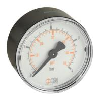
Metal Work pneumatic mechanical pressure gauge, 50mm diameter, 0 to 60 psi, G1/8 male BSPP process connection, center back mount.
