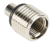
Metal Work hex bushing, G1/4 male BSPP to G1/8 female BSPP, brass. For use with Syntesi Size 2 regulators and filter-regulators.
