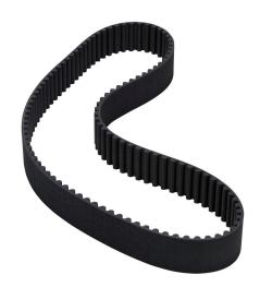
SureMotion timing belt, 8mm 8M pitch, 30mm wide, 110 tooth, 880mm pitch length (circumference), neoprene, fiberglass reinforced.
