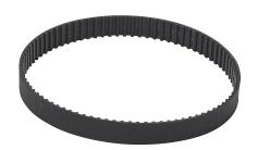
SureMotion timing belt, 0.08in MXL pitch, 1/4in wide, 87 tooth, 7in pitch length (circumference), neoprene, fiberglass reinforced. Package of 3.
