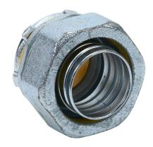
Halex fitting, liquid-tight, malleable iron, straight, 1-1/4in trade size, compression conduit connection, insulation, zinc electroplated finish. Package of 5. For use with LFMC and NM-Type B electrical conduit. Sealing washer and locknut included.
