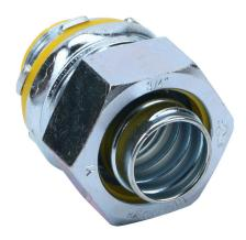
Halex fitting, liquid-tight, malleable iron, straight, 3/4in trade size, compression conduit connection, insulation, zinc electro-plated finish. Package of 5. For use with LFMC and NM-Type B electrical conduit. Sealing washer and locknut included.
