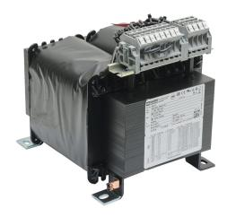
Murrelektronik control transformer, open core, 5 kVA, 1-phase, 208/230/380/400/420/440/460/480/500/525/550 VAC primary, 115/230 VAC secondary, 50/60 Hz, electrostatic shield, panel mount.
