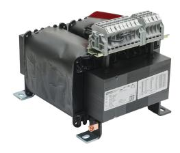
Murrelektronik control transformer, open core, 3 kVA, 1-phase, 208/230/380/400/420/440/460/480/500/525/550 VAC primary, 115/230 VAC secondary, 50/60 Hz, electrostatic shield, panel mount.
