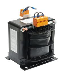
Murrelektronik control transformer, open core, 2.5 kVA, 1-phase, 208/230/380/400/420/440/460/480/500/525/550 VAC primary, 115/230 VAC secondary, 50/60 Hz, electrostatic shield, panel mount.
