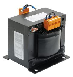
Murrelektronik control transformer, open core, 2 kVA, 1-phase, 208/230/380/400/420/440/460/480/500/525/550 VAC primary, 115/230 VAC secondary, 50/60 Hz, electrostatic shield, panel mount.
