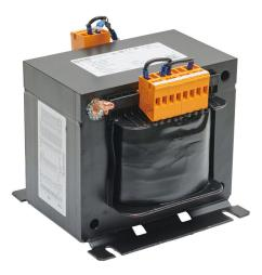
Murrelektronik control transformer, open core, 1.6 kVA, 1-phase, 208/230/380/400/420/440/460/480/500/525/550 VAC primary, 115/230 VAC secondary, 50/60 Hz, electrostatic shield, panel mount.
