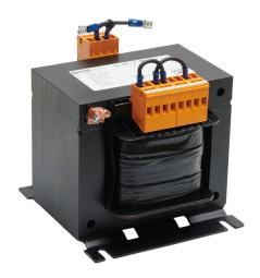
Murrelektronik control transformer, open core, 800 VA, 1-phase, 208/230/380/400/420/440/460/480/500/525/550 VAC primary, 115/230 VAC secondary, 50/60 Hz, electrostatic shield, panel mount.
