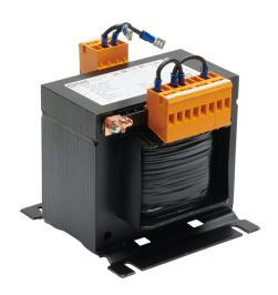
Murrelektronik control transformer, open core, 500 VA, 1-phase, 208/230/380/400/420/440/460/480/500/525/550 VAC primary, 115/230 VAC secondary, 50/60 Hz, electrostatic shield, panel mount.
