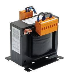
Murrelektronik control transformer, open core, 400 VA, 1-phase, 208/230/380/400/420/440/460/480/500/525/550 VAC primary, 115/230 VAC secondary, 50/60 Hz, electrostatic shield, panel mount.
