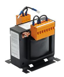
Murrelektronik control transformer, open core, 250 VA, 1-phase, 208/230/380/400/420/440/460/480/500/525/550 VAC primary, 115/230 VAC secondary, 50/60 Hz, electrostatic shield, panel mount.
