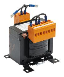
Murrelektronik control transformer, open core, 160 VA, 1-phase, 208/230/380/400/420/440/460/480/500/525/550 VAC primary, 115/230 VAC secondary, 50/60 Hz, electrostatic shield, panel or 35mm DIN rail mount.
