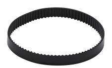
SureMotion timing belt, 0.08in MXL pitch, 1/4in wide, 85 tooth, 6.8in pitch length (circumference), polyurethane, polyester reinforced. Package of 3.
