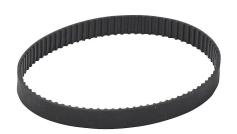
SureMotion timing belt, 0.08in MXL pitch, 1/4in wide, 85 tooth, 6.8in pitch length (circumference), neoprene, fiberglass reinforced. Package of 3.
