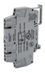
WAGO DC to DC converter, 10-30 VDC input, 10 VDC output, 0.5A, 5W, plastic housing, 35mm DIN rail mount, cage clamp.
