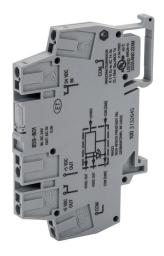
WAGO DC to DC converter, 10-30 VDC input, 5 VDC output, 0.5A, 2.5W, plastic housing, 35mm DIN rail mount, cage clamp.
