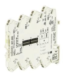
WAGO temperature transmitter, isolated, Input: 1-channel, RTD/potentiometer, deg F or deg C, Output: 1-channel, current/voltage, 24 VDC operating voltage, 35mm DIN rail mount, pushin terminals, hazardous location rated.
