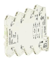
WAGO signal conditioner, isolated, Input: 1-channel, current, 4-20 mA, Output: 1-channel, voltage, 0-10 VDC, 24 VDC operating voltage, 35mm DIN rail mount.
