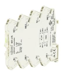
WAGO signal conditioner, isolated, Input: 1-channel, current, 0-20 mA, Output: 1-channel, voltage, 0-10 VDC, 24 VDC operating voltage, 35mm DIN rail mount.
