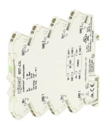
WAGO signal conditioner, isolated, Input: 1-channel, voltage, 0-10 VDC, Output: 1-channel, current, 4-20 mA, 24 VDC operating voltage, 35mm DIN rail mount.
