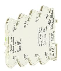
WAGO signal conditioner, isolated, Input: 1-channel, voltage, 0-10 VDC, Output: 1-channel, current, 0-20 mA, 24 VDC operating voltage, 35mm DIN rail mount.
