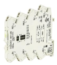
WAGO signal conditioner, isolated, Input: 1-channel, current/voltage, Output: 1-channel, current/voltage, 24 VDC operating voltage, 35mm DIN rail mount.
