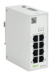
WAGO industrial lean managed Ethernet switch, MAC Security, 8 ports, (8) Ethernet Gigabit (RJ45) port(s), Modbus TCP and SNMP, -20 to +70 deg C, metal housing, IP30, 35mm DIN rail mount.
