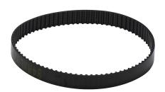
SureMotion timing belt, 0.08in MXL pitch, 1/4in wide, 84 tooth, 6.7in pitch length (circumference), polyurethane, polyester reinforced. Package of 3.
