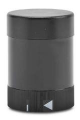
WERMA buzzer element, 80 dB at 1m, 21 kHz tone frequency, continuous/pulse tone(s), 115 VAC/VDC, ABS/polycarbonate housing, black, IP54. For use with WERMA 50mm stack light elements.
