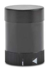
WERMA buzzer element, 80 dB at 1m, 21 kHz tone frequency, continuous/pulse tone(s), 24 VAC/VDC, ABS/polycarbonate housing, black, IP54. For use with WERMA 50mm stack light elements.
