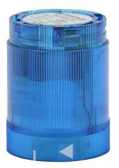
WERMA LED light element, 50mm diameter, blue, flashing (1 Hz ON for 10ms) light function, 24 VDC, colored lens, IP54.
