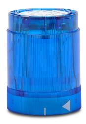
WERMA LED light element, 50mm diameter, blue, blinking (1 Hz ON for 550ms) light function, 24 VAC/VDC, colored lens, IP54.
