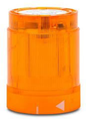
WERMA LED light element, 50mm diameter, yellow, blinking (1 Hz ON for 550ms) light function, 24 VAC/VDC, colored lens, IP54.
