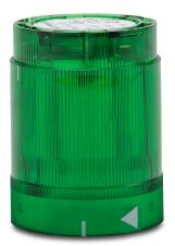
WERMA LED light element, 50mm diameter, green, blinking (1 Hz ON for 550ms) light function, 24 VAC/VDC, colored lens, IP54.
