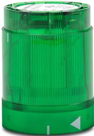
WERMA LED light element, 50mm diameter, green, permanent light function, 24 VAC/VDC, colored lens, IP54.
