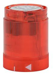
WERMA LED light element, 50mm diameter, red, flashing (1 Hz ON for 10ms) light function, 24 VDC, colored lens, IP54.
