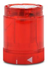
WERMA LED light element, 50mm diameter, red, blinking (1 Hz ON for 550ms) light function, 24 VAC/VDC, colored lens, IP54.
