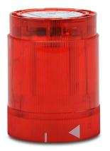
WERMA LED light element, 50mm diameter, red, permanent light function, 115 VAC, colored lens, IP54.
