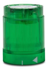
WERMA incandescent light element, 50mm diameter, green, permanent light function, 12-240 VAC/VDC, colored lens, IP54. Requires incandescent bulb.
