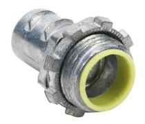
Halex fitting, zinc die cast, straight, 1/2in trade size, screw-in conduit connection, insulation. Package of 50. For use with flexible metal conduit (FMC). Locknut included.
