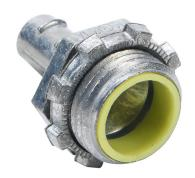
Halex fitting, zinc die cast, straight, 3/8in trade size, screw-in conduit connection, insulation. Package of 50. For use with flexible metal conduit (FMC). Locknut included.
