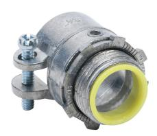
Halex fitting, zinc die cast, straight, 3/4in trade size, squeeze conduit connection, insulation. Package of 25. For use with flexible metal conduit (FMC), AC cable (BX), MC cable. Screw and locknut included.
