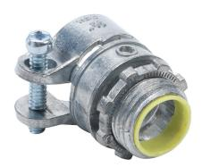
Halex fitting, zinc die cast, straight, 1/2in trade size, squeeze conduit connection, insulation. Package of 25. For use with flexible metal conduit (FMC), AC cable (BX), MC cable. Screw and locknut included.
