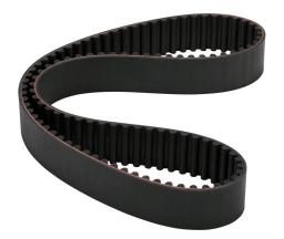
SureMotion timing belt, 8mm 8M pitch, 30mm wide, 105 tooth, 840mm pitch length (circumference), neoprene, fiberglass reinforced.
